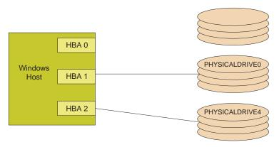
The default driver behavior does not store target bindings between host reboots. The bindings are dynamically generated by the HBA when new target devices are detected.
